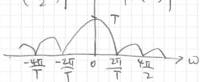
This has lowpass filtering effect. BW of filter  $\approx \frac{1}{T}$  Hz.
