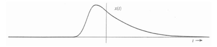
• Example of a signal with finite power, which implies that the energy of the signal is infinite.
