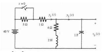
Initial conditions:  $y_1(0^-) = 4 A$ ,  $y_2(0^-) = 0 A$ ,  $v_0(0^-) = 16 V$
