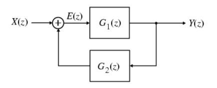
• Eliminating E(z) from the previous two equations we arrive at  $[1 - G_1(z)G_2(z)]Y(z) = G_1(z)X(z)$
