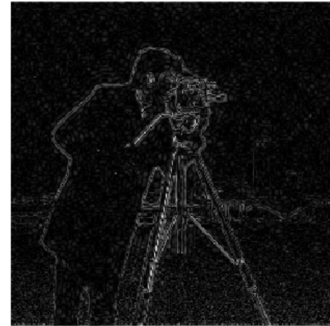
Figure 27: Corresponding error image for Figure 26 ( |\text{original} - \text{restored}| , scaled for display)
