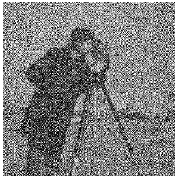
Figure 30: CLS restoration of Figure 3 with \alpha = 0.0001 , ISNR = -21.5 Figure 44: CLS restoration of Figure 5 with \alpha = 0.0001 , ISNR = -22.1 dB
