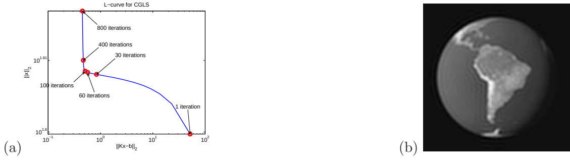
Figure 5.9: (a) L-curve; (b) Super-resolved image with Conjugate Gradient algorithm and L-curve method: PSNR = 23.8 dB. The corner of the L-curve is achieved at 100 iterations approximately.
