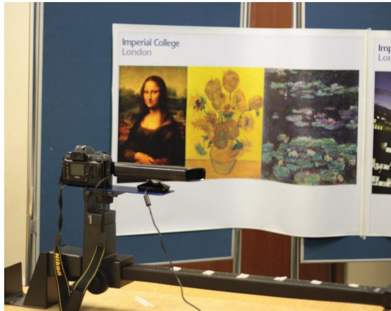
**Figure 6.2:** Acquisition rig for capturing high resolution simultaneous RGB-D images along an EPI line.
