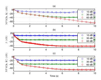
Fig. 2. (a) NPM between true and estimated systems, (b) Cost function, (c) NPM between true and channel-dependent component of estimated system for random channels with varying SNR.
