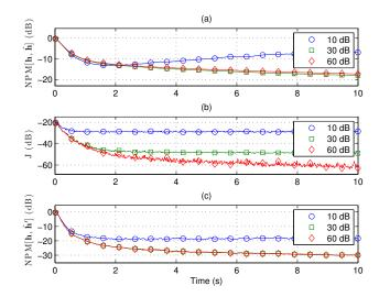
Fig. 1. (a) NPM between true and estimated systems, (b) Cost function, (c) NPM between true and channel-dependent component of estimated system for room impulse responses with varying SNR.
