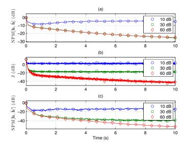
Fig. 3. (a) NPM between true and estimated systems, (b) Cost function, (c) NPM between true and channel-dependent component of estimated system for exponentially-decaying random channels with varying SNR.
