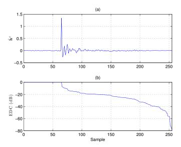
Fig. 5. (a) Common component for a misconverged system, (b) Energy decay curve of the common component.
