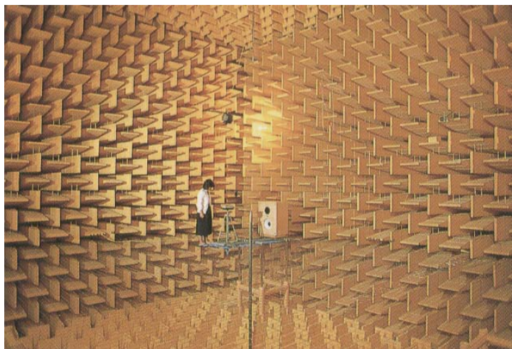
Figure 2.5: A loudspeaker is placed inside an anechoic chamber, which absorbs most of the radiated sound energy, allowing the frequency response of the loudspeaker to be accurately measured. Depicted is a particularly large chamber at NMIJ in Japan.
