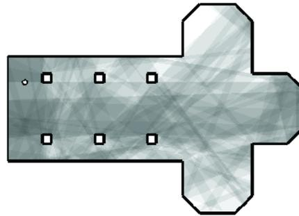
Fig. 2: Superposition of beams in a complex 2D environment (only reflections up to the 2<sup>nd</sup> order are visualized).
