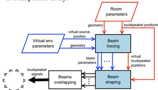
Fig. 1: Block diagram of a geometric WFS engine.
