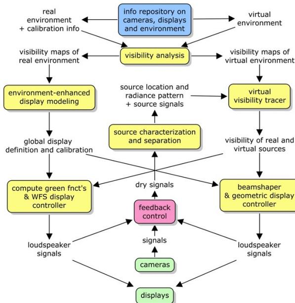
Fig. 7: Wavefield rendering: combining Wavefield Synthesis methods with Geometric Rendering methodologies.
