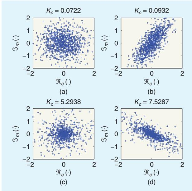
**[FIG2]** Circularity plots for complex doubly white noises. (a) circular Gaussian, (b) noncircular Gaussian ( $\eta = 0.81$ ), (c) circular Laplacian noise, and (d) noncircular Laplacian ( $\eta = 0.81$ ). Symbol  $K_c$  denotes the kurtosis.
