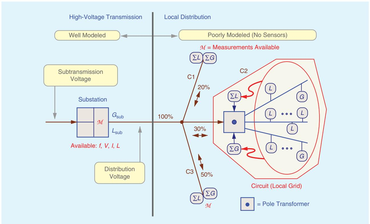
**[FIG1] Nodal estimation.** Various loads (L) and small generators (G) operate locally and contribute to the variability of power quality. A substation has three to five circuits. The sum of all the circuit loads  $\Sigma L$  and all the generation  $\Sigma G$  equals that of the substation. A G-L mismatch in one circuit is compensated from the generation in another circuit or from the main grid.
