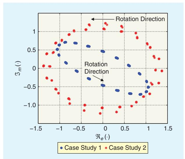
**[FIG11]** Noncircularity of real world unbalanced voltage sags.
