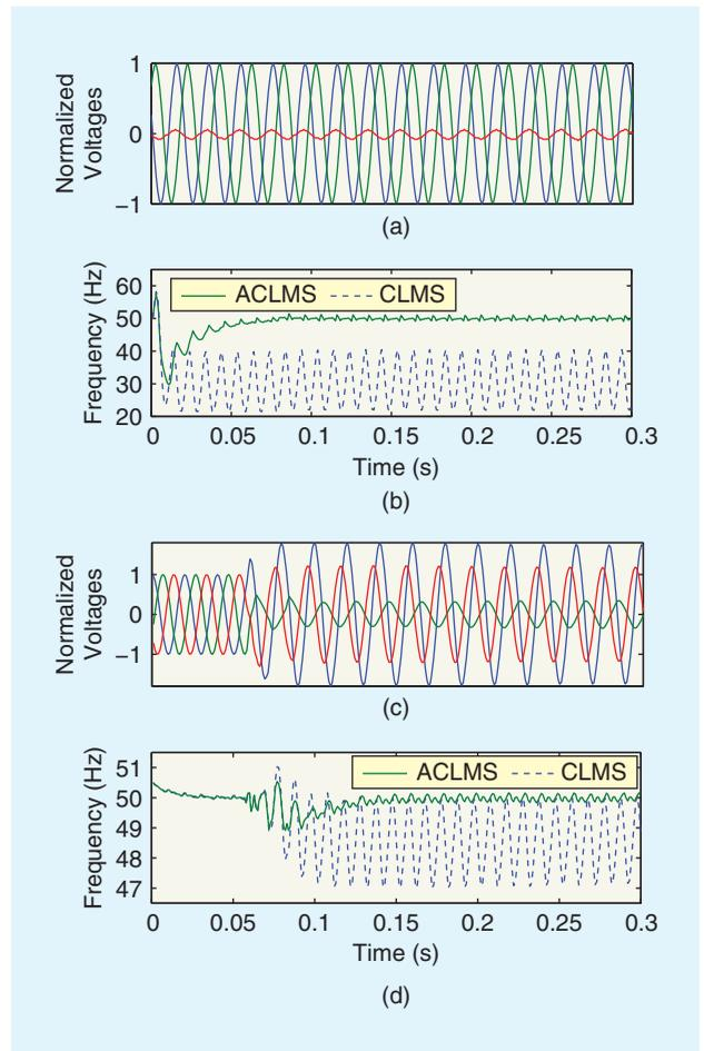
**[FIG10]** Frequency estimation for real-world voltage sags. (a) Phase C undergoes a voltage dip of 94%, (b) frequency estimation using CLMS (broken) and ACLMS (solid), (c) Phase B experiences a short circuit and Phase A and Phase C go into a swell, and (d) frequency estimation using CLMS (broken) and ACLMS (solid).
