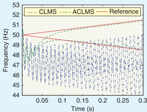
**[FIG8]** Estimation for a mismatch between generation and consumption (frequency rise and decay). The widely linear ACLMS approached the correct value to within 5% in 50 ms.
