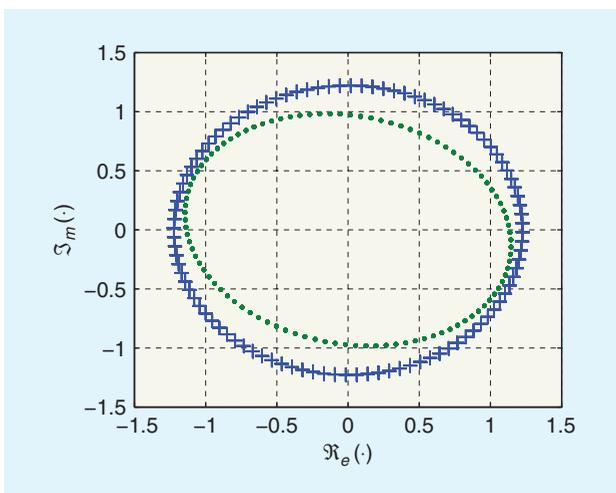
**[FIG3]** Circularity via the "real-imaginary" ( $\Re - \Im$ ) scatter plot. The blue circle denoted by "+" corresponds to a circular  $v(k)$  in a balanced system ( $V_a(k) = V_b(k) = V_c(k)$ ) at 1 per unit (p.u.). The green ellipse denoted by "." corresponds to a noncircular  $v(k)$  stemming from an unbalanced system with  $V_a(k) = 1$  p.u.,  $V_b(k) = 0.9$  p.u., and  $V_c(k) = 0.7$  p.u.
