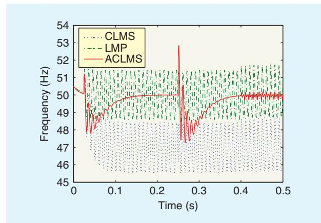
**[FIG7] Frequency estimation for a cascade of harmful events: strictly linear CLMS and LMP versus widely linear ACLMS.**
