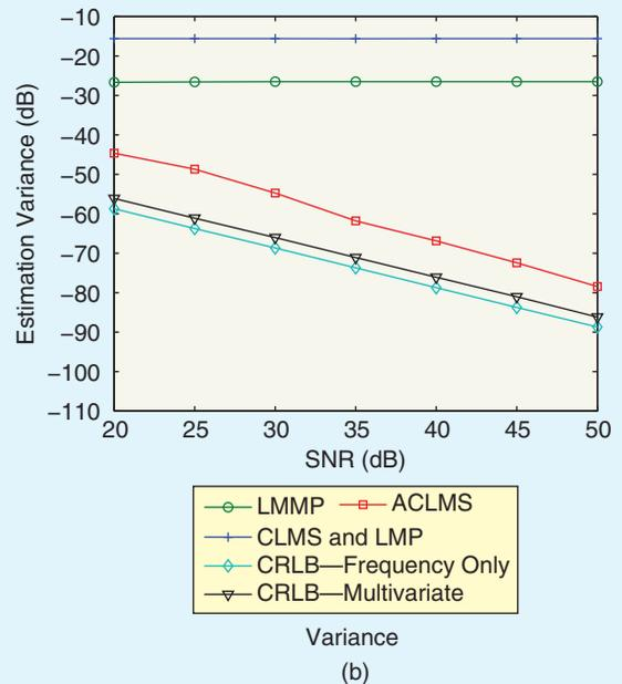
**[FIG9]** Bias and variance of the widely linear ACLMS, and the strictly linear CLMS, LMP, and LMMP compared to CRLB (curves averaged over 1,000 independent trials). (a) Bias: the widely linear ACLMS is asymptotically unbiased, followed by LMP and (b) variance: the widely linear ACLMS is a consistent estimator.
