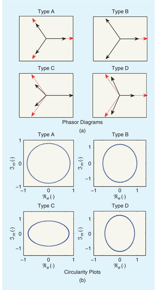
**[FIG5] Unbalanced voltage sags due to single phase-to-ground faults, for the characteristic voltage of  $V = 0.7$ . (a) Phasor diagram (dotted line denotes balanced operation) and (b) circularity via a “real-imaginary” plot.**
