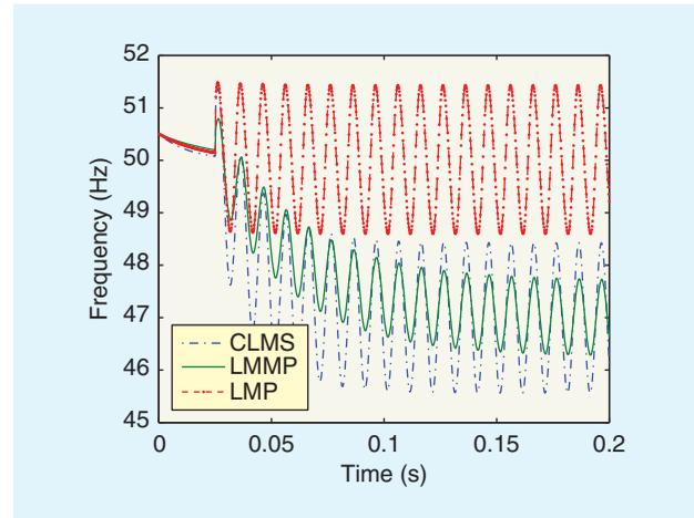
**[FIG6] Frequency estimation for Type C voltage sag.**
