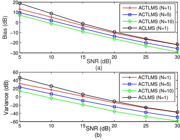
Fig. 1. Statistical evaluation of the considered frequency estimation methods for a noisy unbalanced power system against different SNRs. (a) Bias. (b) Variance.
