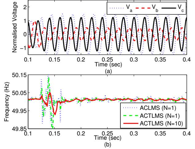
Fig. 3. Frequency estimation using the proposed ACTLMS based algorithms for a real-world unbalanced three-phase power system. (a) The waveform of the three-phase power system. (b) Comparison of frequency estimation results by the considered methods.
