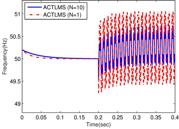
Fig. 2. Performance comparison of the proposed ACTLMS algorithm for different filter lengths,  $N$ .
