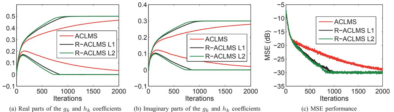
Fig. 2. Coefficient convergence of the ACLMS and R-ACLMS for a strictly linear system with a noncircular input signal.
