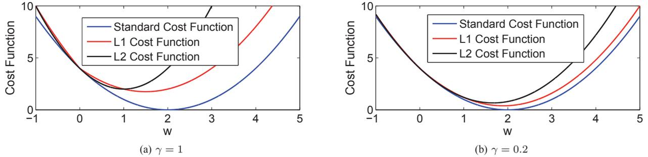
Fig. 1. Comparison between the  $l_1$ - and  $l_2$ -norm regularised cost functions for different values of  $\gamma$ . The standard cost function is achieved by setting  $\gamma = 0$ .
