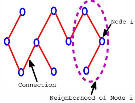
Fig. 1. A distributed network with  $N = 10$  nodes.
