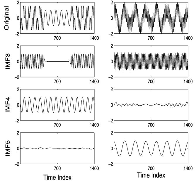
Fig. 7. Decomposition of a synthetic bivariate tone signal via noise-assisted MEMD for  $m = 2$ . Both the problems of mode mixing and mode misalignment are clearly reduced. Again, the obtained results were generally found robust to variations in the parameters.
