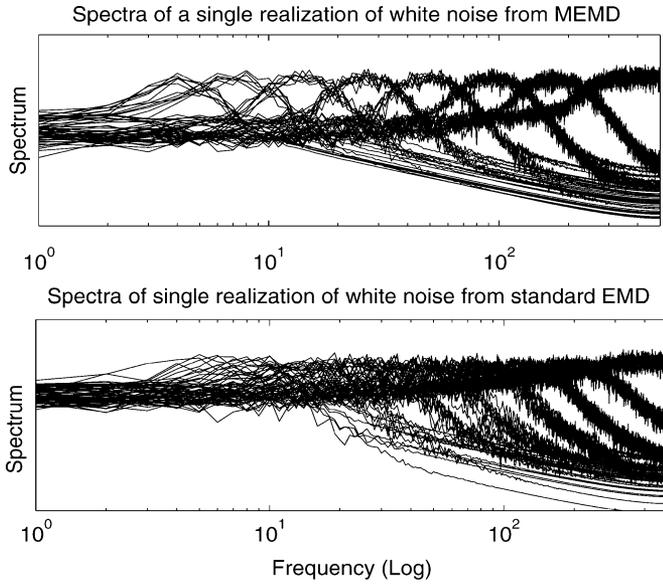
Fig. 1. Spectra of IMFs (IMF1-IMF9) obtained for a single realization of an eight-channel white Gaussian noise via MEMD (top) and the standard EMD (bottom). Overlapping of the frequency bands corresponding to the same-index IMFs is more prominent in the case of MEMD based filters.
