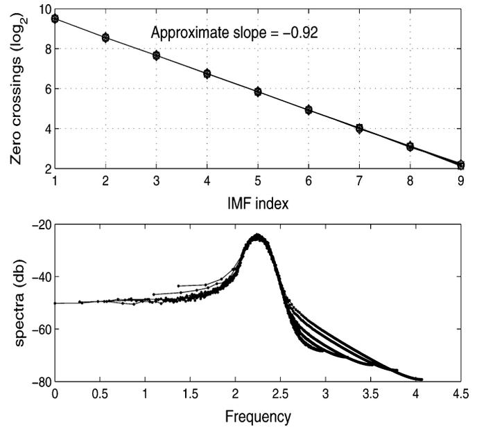
Fig. 3. MEMD as a dyadic filter bank. Top: Average number of base-2 logarithm of zero crossings plotted versus the IMF index for all eight channels. The slope of  $-0.92$  indicates similarity to a dyadic filter (with an ideal slope  $-1$ ). Bottom: Fourier spectra of IMFs from MEMD with IMF3-IMF9 shifted so as to overlap with the spectrum associated with IMF2.
