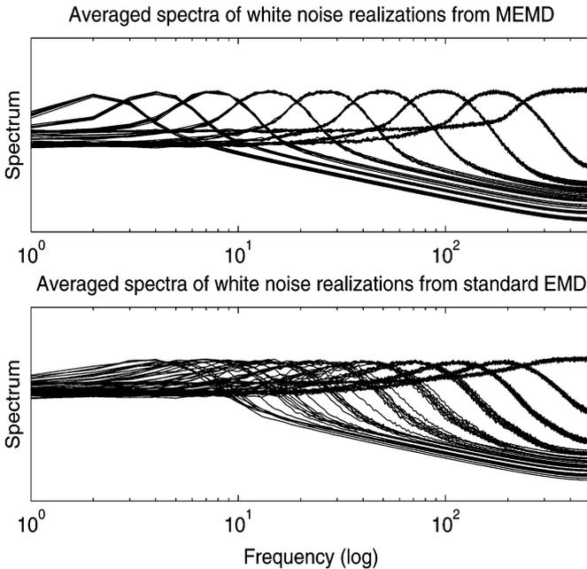
Fig. 2. Averaged spectra of IMFs (IMF1-IMF9) obtained for a  $N = 500$  realizations of eight-channel white Gaussian noise via MEMD (top) and the standard EMD (bottom). Overlapping of the frequency bands corresponding to the same-index IMFs is improved in both cases but the MEMD bands clearly show much better alignment.
