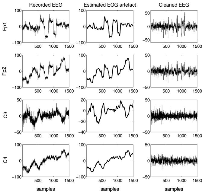
Fig. 8. Artefact removal from four EEG channels ( $Fp1$ ,  $Fp2$ ,  $C3$  and  $C4$ ) using the MEMD algorithm. The estimated eye muscle activity (artefact) has been shown in the middle column, whereas the conditioned EEG signal is presented in the right hand column.
