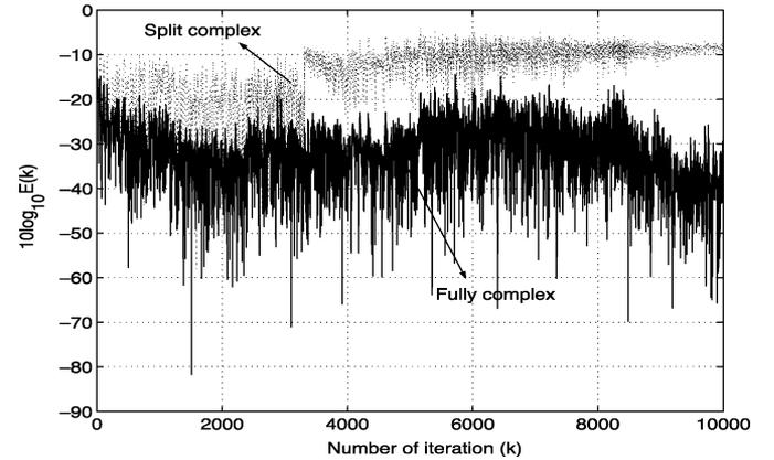
Fig. 7. Performance curve of fully CRTRL and split CRTRL for radar signal.
