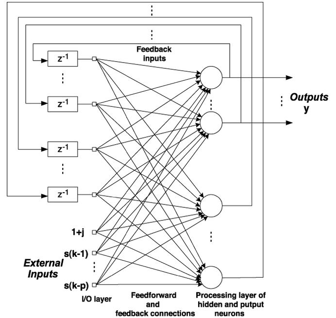
Fig. 1. Fully connected recurrent neural network for prediction.
