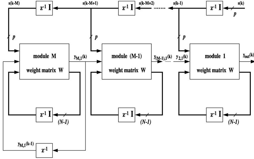
Fig. 2. Pipelined Recurrent Neural Network (PRNN).
