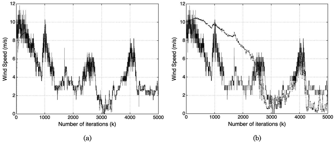
Fig. 8. Prediction of complex wind signal using CPRNN+FIR. Solid curve: actual wind signal. Dashed curve: nonlinear prediction. (a) Performance based on fully complex activation function; (b) performance based on split complex activation function.
