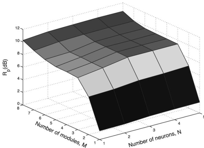
Fig. 4. Relationship between prediction gain  $R_p$ , number of modules  $M$ , and number of neurons  $N$  for nonlinear prediction of the complex wind signal.
