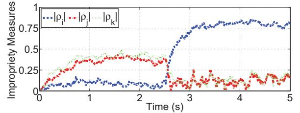
Fig. 5. Channel improbity measure estimation of an Alamouti communication system.
