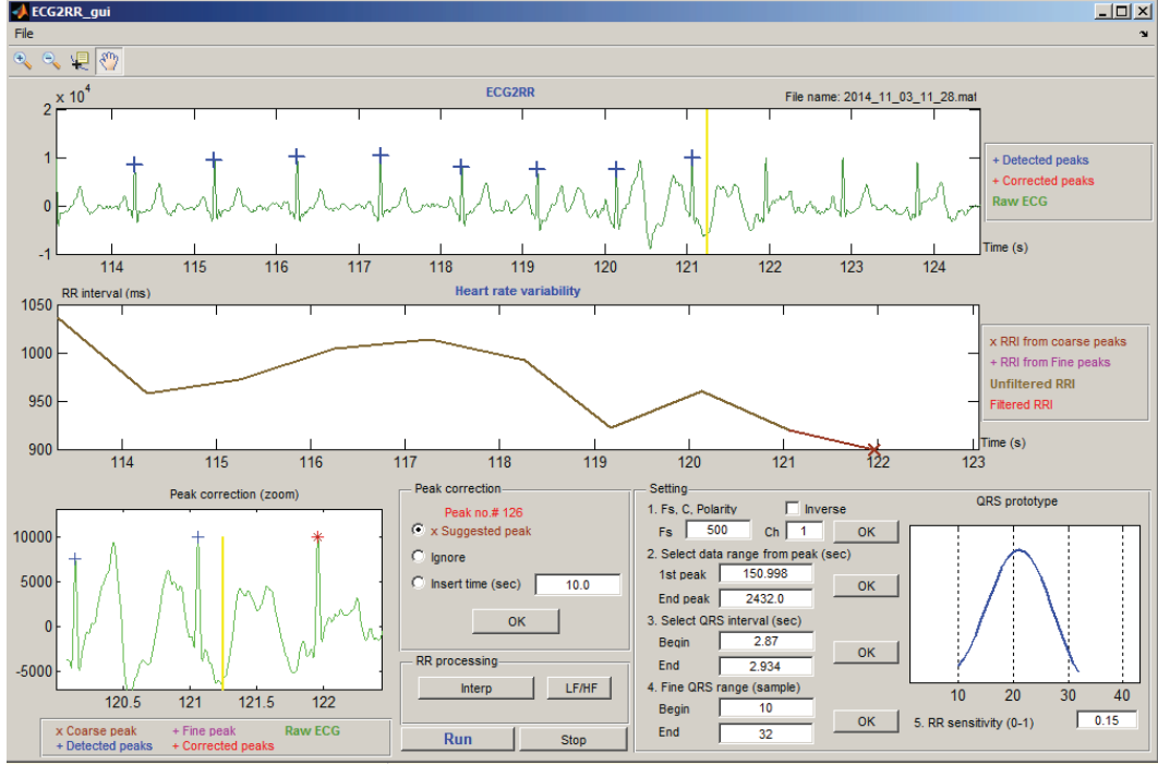
Fig. 3. Software for R-peak extraction using the MF-HT algorithm. Four windows are designed to visualise: ECG and identified R-peaks, the RR-intervals, a close-up R-peak examination with suggested choices, and the QRS pattern selection and settings.
