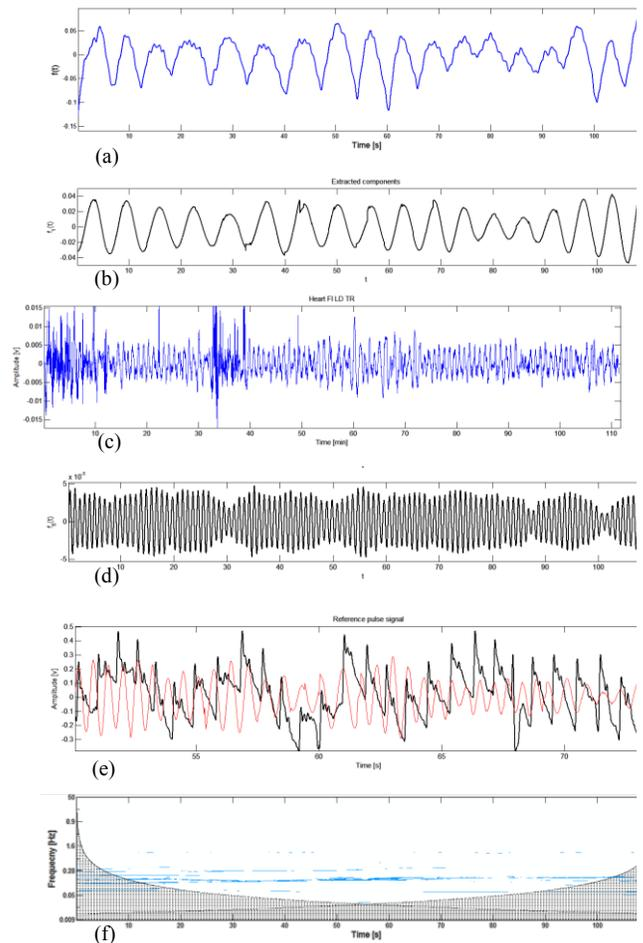
Figure 6. Experimental results (a) Radar baseband output contains both respiration and heart signal; (b) First extracted oscillating component which represent respiration signal; (c) Heart signal after bandpass filtering; (d) Fifth extracted oscillating component which represent heart signal. (e) extracted fifth component versus reference finger pulse for heart signal; (f) Synchrosqueezed output
