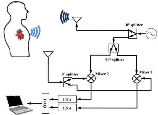
Figure 5. Doppler radar quadrature receiver experimental setup
