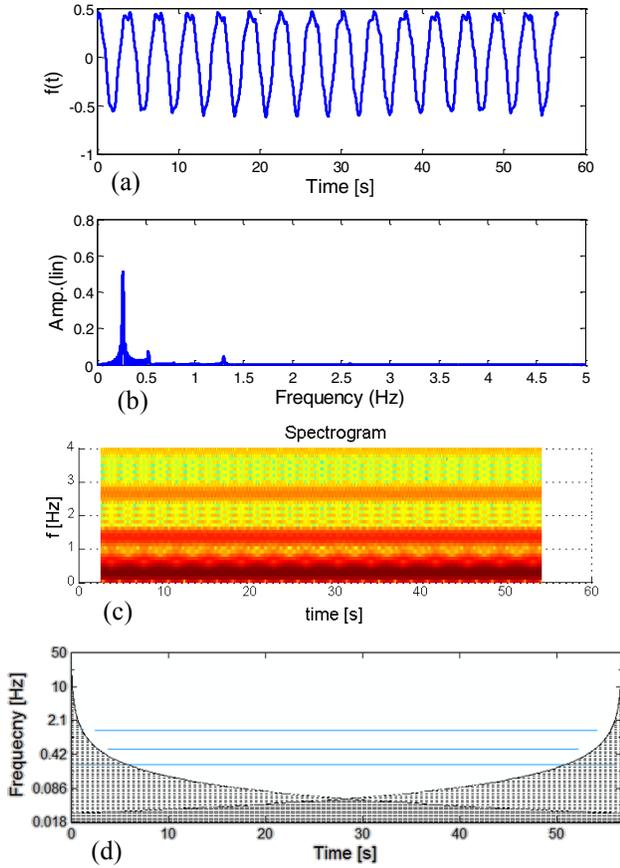
Figure 3. (a) Heart and respiration complex signal; (b) Spectrum of the signal; (c) Spectrogram; (d) Synchrosqueezed output.
