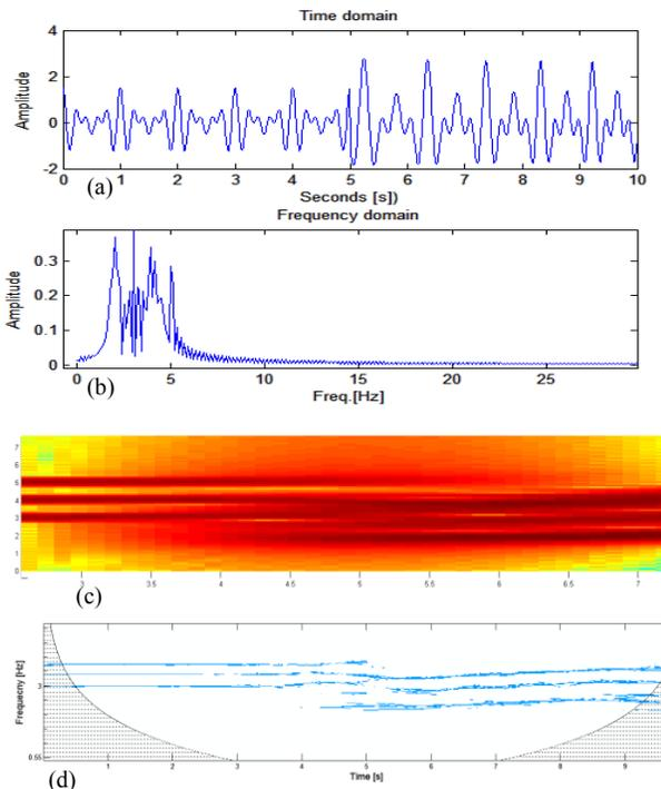
Figure 2. A more complex signal for performance comparison; (a) time-domain signal  $s(t)$ ; (b) Spectrum of the signal; (c) Spectrogram; (d) Synchrosqueezed output.
