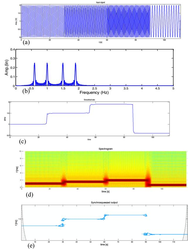
Figure 1. Comparison of Synchrosqueezing with DFT method and Spectrogram; (a) time-domain signal  $s(t)$ ; (b) Spectrum of the signal; (c) DFT rate; (d) Spectrogram (e) Synchrosqueezed output.
