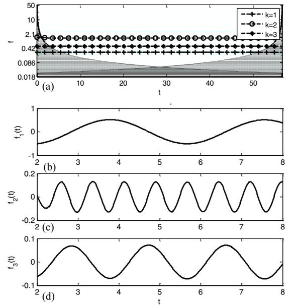
Figure 4. (a) Synchrosqueezed output with marked components of TF plot; (b)(c)(d) First three components of the complex signal
