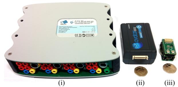
**FIGURE 5. The three recording devices used: (i) g.USBamp by g.tec; (ii) Avatar by EGI; and (iii) our own custom-made recorder with a 24 bit ADC. For reference, the devices are pictured against a 20 pence coin.**
