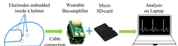
**FIGURE 6. The final setup: Electrodes inside the helmet (and reference electrodes) are attached to a biosignal-amplifier which writes data to an SD-card. The SD-card can be replaced with a Bluetooth adapter.**
