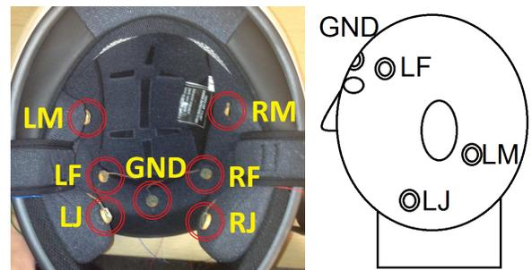
Fig. 1. Setup of the helmet (left) and the positions of the electrodes on the head (right).
