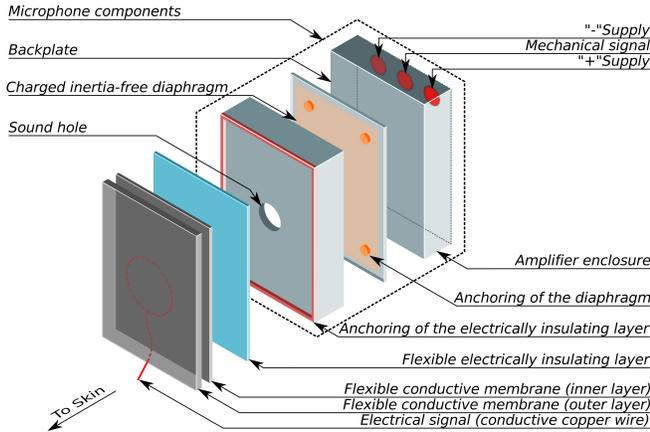
Fig. 1. Detailed construction diagram of the multimodal sensor.
