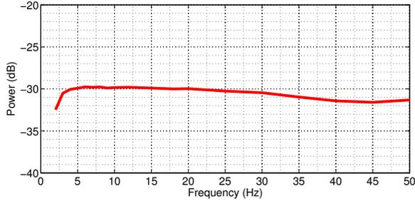
Fig. 3. Frequency response of the mechanical part of the multimodal sensor. The sensor was firmly attached to the vibration plate oscillating at a 1 mm displacement amplitude and the frequency was varied over a 2 – 50Hz range.
