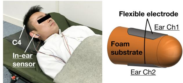
Fig. 2. Left: Recording setup. The electrodes were placed on scalp and in the ear canal. The subject seated and reclined in a comfortable chair. Right: The wearable viscoelastic in-ear sensor with two flexible electrodes [22].
