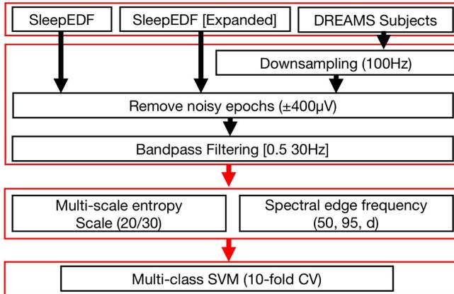
Fig. 4. Flowchart of an automatic sleep staging system
