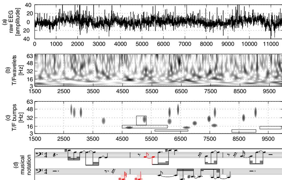
**Fig. 3.** An example of TF domain bumps modeling for EEG sonification. The above diagrams present: (a) The original raw EEG signal captured during a steady state visual evoked paradigm experiment; (b) wavelets representation the above EEG signal; (c) sparse bump modeling procedure of the above wavelets; (d) is a translation of obtained MIDI representation into classical musical sheet.
