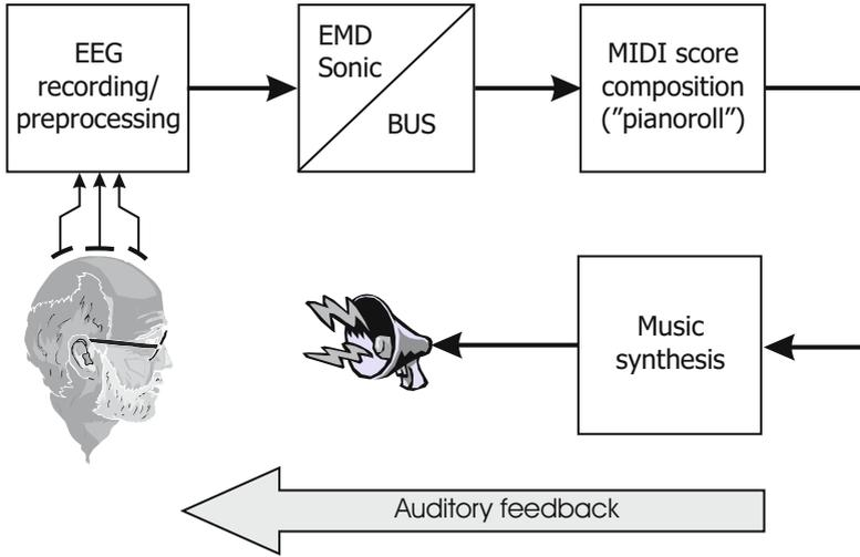
**Fig. 1.** Block diagram of the proposed EEG sonification scheme for brain computer interfaces. An auditory feedback i.e. a mapping from EEG features onto a discrete set of musical variables, provides a convenient insight into the dynamics and patterns of EEG events.
