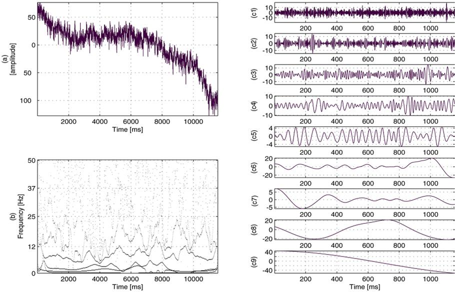
**Fig. 2.** An example of EEG signal decomposition using EMD technique. Clockwise from top left panel: (a) Raw EEG signal recorded from single frontal (Fp1) electrode. The panels (c1)-(c9) present nine IMF components extracted sequentially. IMFs represent oscillations occurring in EEG from higher to lower frequencies. (b) The oscillatory components ranging from 1Hz to 50Hz are combined in form of Hilber-Huang spectrum [9].
