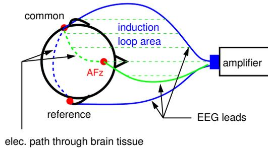
Fig. 3. Induction loops causing magnetic interference.
