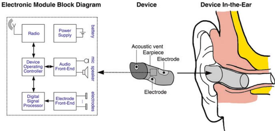
**Fig. 4** An illustration of a future Ear-EEG device with an electronic module comprising instrumentation for the electrode signals, analog-to-digital conversion, a signal processing unit, battery, and a radio module
