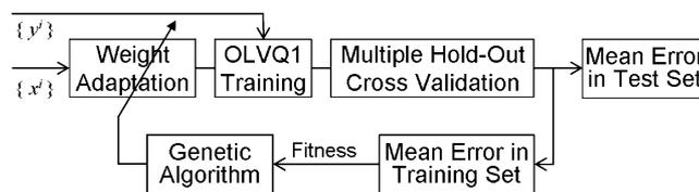
Figure 2. Scheme of our proposed feature weighting system utilizing OLVQ1 as classification method and a genetic algorithm as optimization method. Mean empirical training errors are used as fitness measure.
