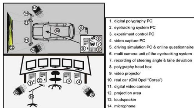
Figure 1. Real car driving simulation lab.
