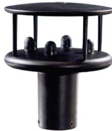
(e) Gill Inst. 2D ultrasonic anemometer
