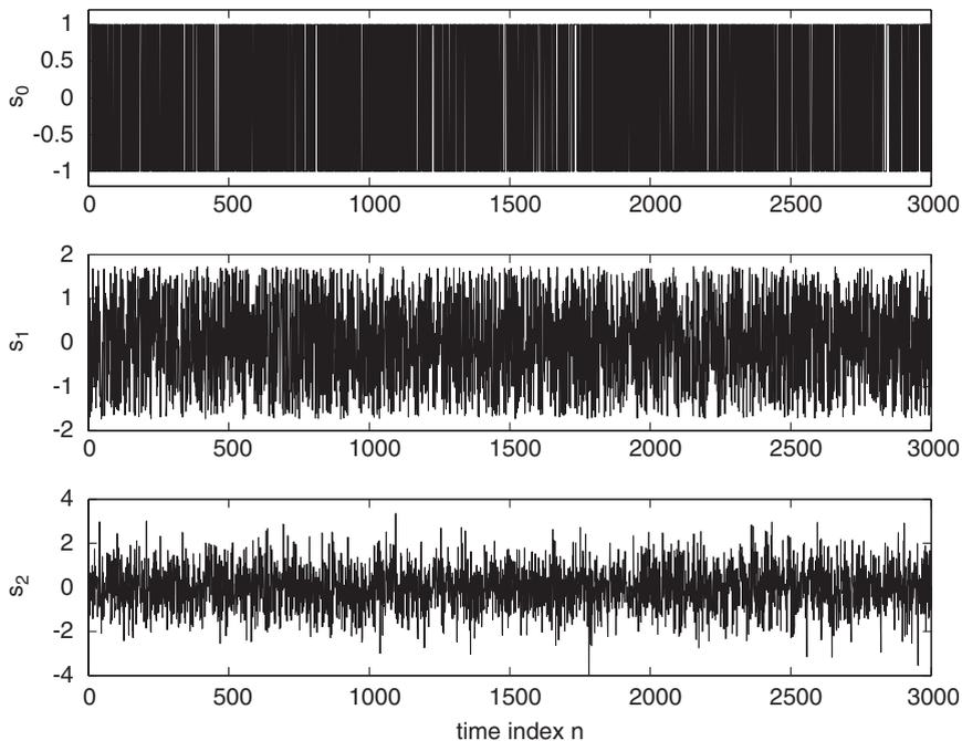
Fig. 1. The three source signals with binary, uniform and Gaussian distributions, respectively.
