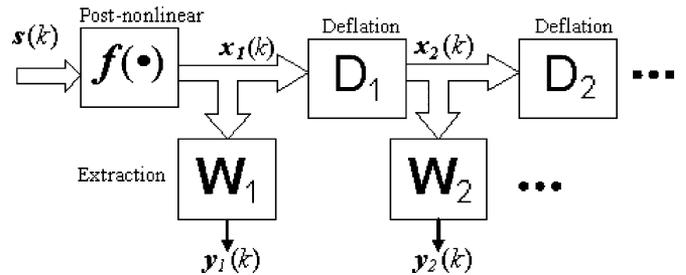
Fig. 2. General structure of the blind source extraction (BSE).
