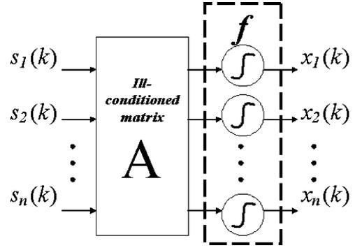
Fig. 1. Block diagram of the ill-conditioned post-nonlinear mixing model.
