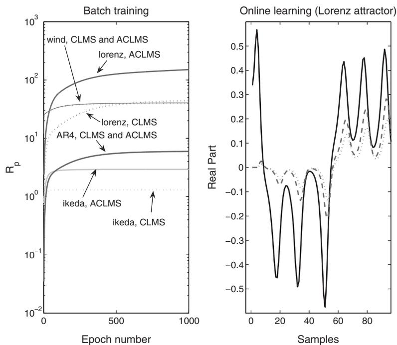
**Figure 13.2** Comparison of the ACLMS and standard CLMS. Left: Prediction gains  $R_p$  for signals DS1 – DS4. Right: Tracking performance for the Lorenz signal; solid line represents the original signal, dotted line the CLMS based prediction, and dashed line the ACLMS based prediction
