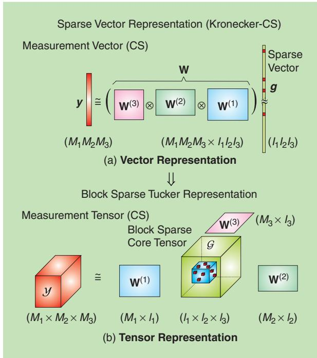
**[FIG7]** CS with a Kronecker-structured dictionary. OMP can perform faster if the sparse entries belong to a small subtensor, up to permutation of the columns of  $\mathbf{W}^{(1)}$ ,  $\mathbf{W}^{(2)}$ , and  $\mathbf{W}^{(3)}$ .
