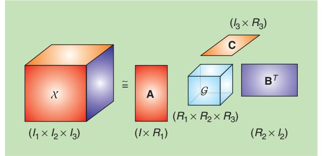
**[FIG4]** The Tucker decomposition of a third-order tensor. The column spaces of  $\mathbf{A}$ ,  $\mathbf{B}$ , and  $\mathbf{C}$  represent the signal subspaces for the three modes. The core tensor  $\mathcal{G}$  is nondiagonal, accounting for the possibly complex interactions among tensor components.
