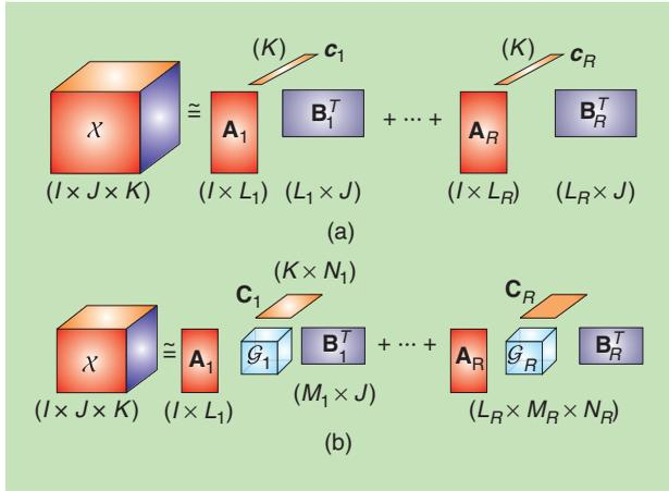
**[FIG5] BTDs find data components that are structurally more complex than the rank-1 terms in CPD. (a) Decomposition into terms with multilinear rank  $(L_r, L_r, 1)$ . (b) Decomposition into terms with multilinear rank  $(L_r, M_r, N_r)$ .**
