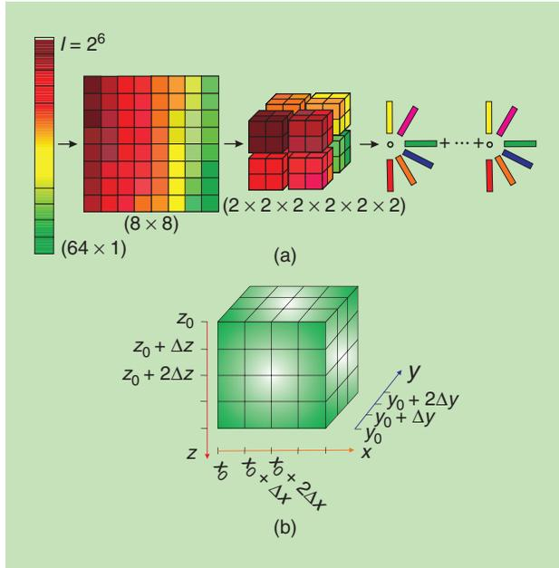
**[FIG2] Construction of tensors. (a) The tensorization of a vector or matrix into the so-called quantized format; in scientific computing, this facilitates supercompression of large-scale vectors or matrices. (b) The tensor is formed through the discretization of a trivariate function  $f(x,y,z)$ .**
