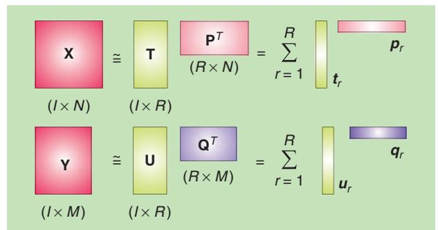
**[FIG12]** The basic PLS model performs joint sequential low-rank approximation of the matrix of predictors  $\mathbf{X}$  and the matrix of responses  $\mathbf{Y}$  so as to share (up to the scaling ambiguity) the latent components—columns of the score matrices  $\mathbf{T}$  and  $\mathbf{U}$ . The matrices  $\mathbf{P}$  and  $\mathbf{Q}$  are the loading matrices for predictors and responses, and  $\mathbf{E}$  and  $\mathbf{F}$  are the corresponding residual matrices.
