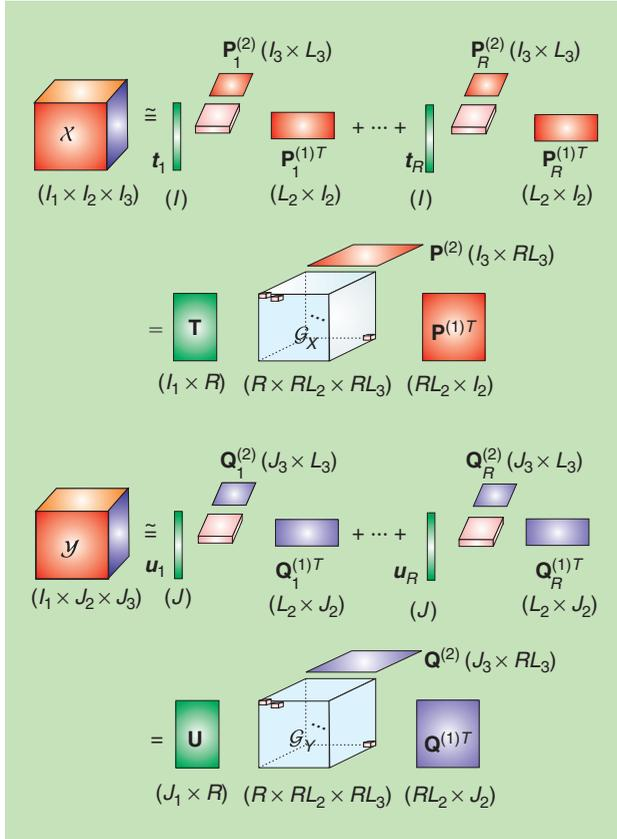
**[FIG13]** The principle of HOPLS for third-order tensors. The core tensors  $\mathcal{G}_X$  and  $\mathcal{G}_Y$  are block-diagonal. The BTD-type structure allows for the modeling of general components that are highly correlated in the first mode.
