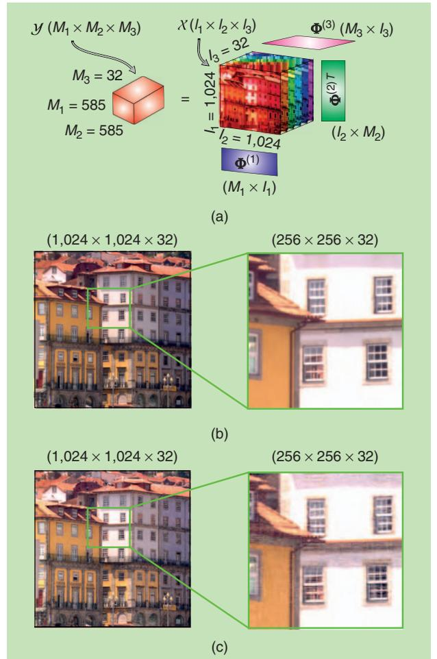
**[FIG8]** The multidimensional CS of a 3-D hyperspectral image using Tucker representation with a small sparse core in wavelet bases. (a) The Kronecker-CS of a 32-channel hyperspectral image. (b) The original hyperspectral image-*RGB* display. (c) The reconstruction (SP = 33%, PSNR = 35.51 dB)-*RGB* display.
