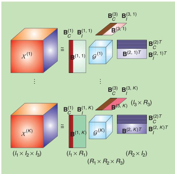
**[FIG15] Coupled TKD for LMWCA.** The data tensors have both shared and individual components. Constraints such as orthogonality, statistical independence, sparsity, and nonnegativity may be imposed where appropriate.
