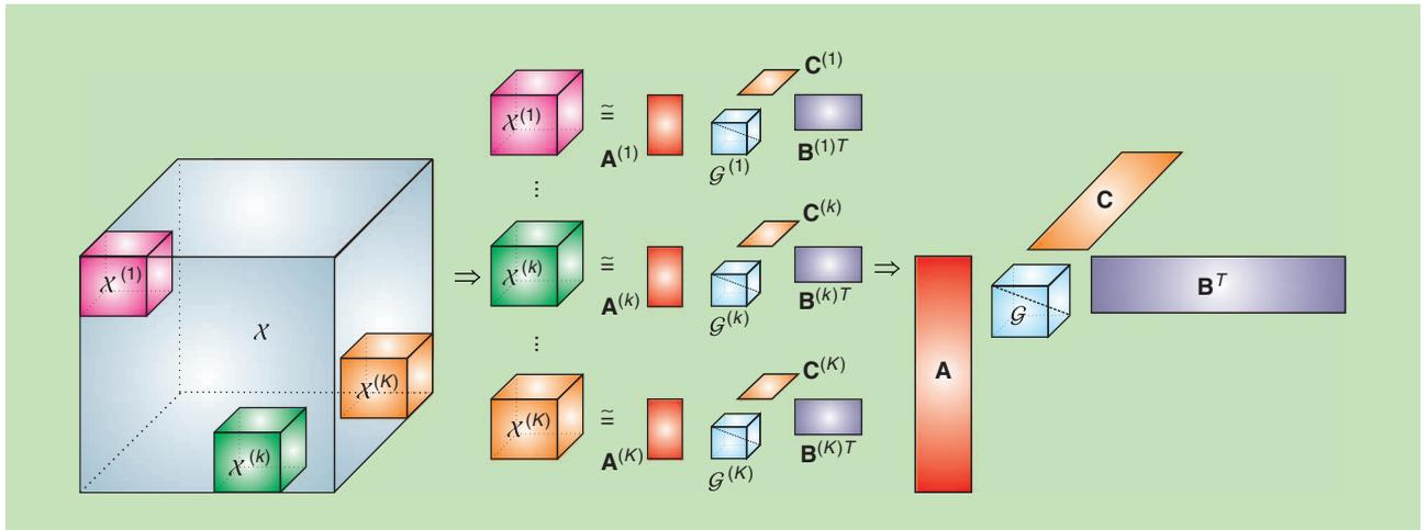
**[FIG10]** Efficient computation of CPD and TKD, whereby tensor decompositions are computed in parallel for sampled blocks. These are then merged to obtain the global components  $\mathbf{A}$ ,  $\mathbf{B}$ , and  $\mathbf{C}$ , and a core tensor  $\mathcal{G}$ .
