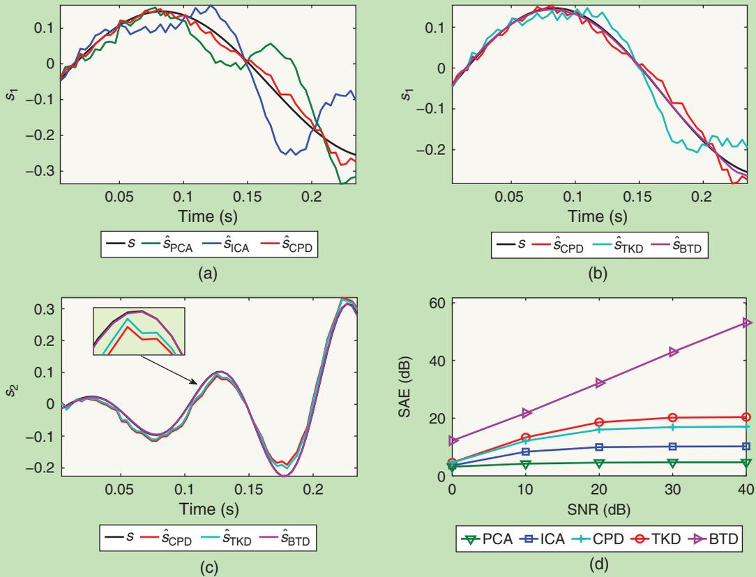
**[FIG6]** The blind separation of the mixture of a pure sine wave and an exponentially modulated sine wave using PCA, ICA, CPD, TKD, and BTD. The sources  $s_1$  and  $s_2$  are correlated and of short duration; the symbols  $\hat{s}_1$  and  $\hat{s}_2$  denote the estimated sources. (a)–(c) Sources  $s_1(t)$  and  $s_2(t)$  and their estimates using PCA, ICA, CPD, TKD, and BTD; (d) average squared angular errors (SAE) in estimation of the sources.
