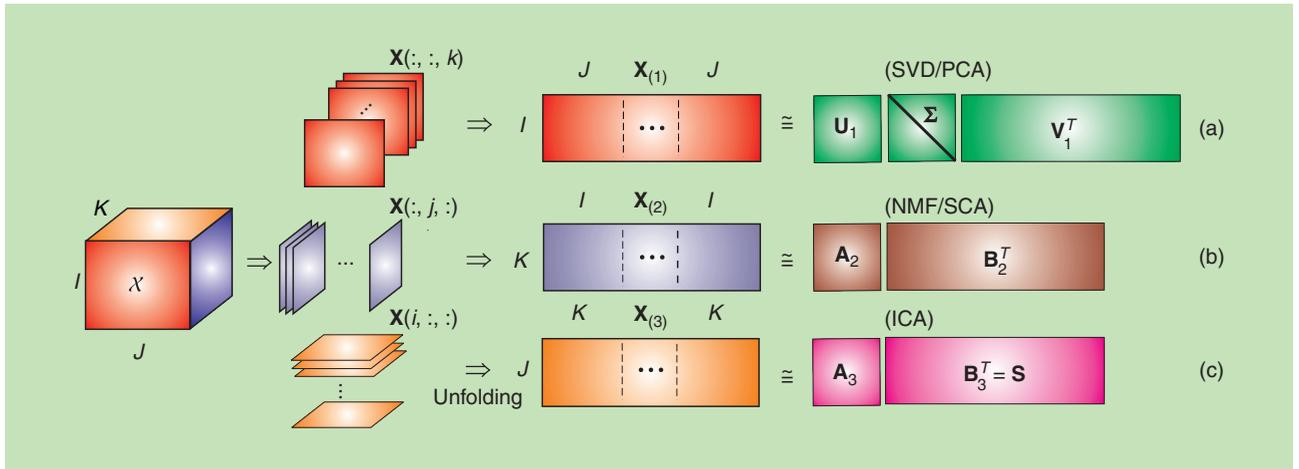
**[FIG1] MWCA for a third-order tensor, assuming that the components are (a) principal and orthogonal in the first mode, (b) nonnegative and sparse in the second mode, and (c) statistically independent in the third mode.**
