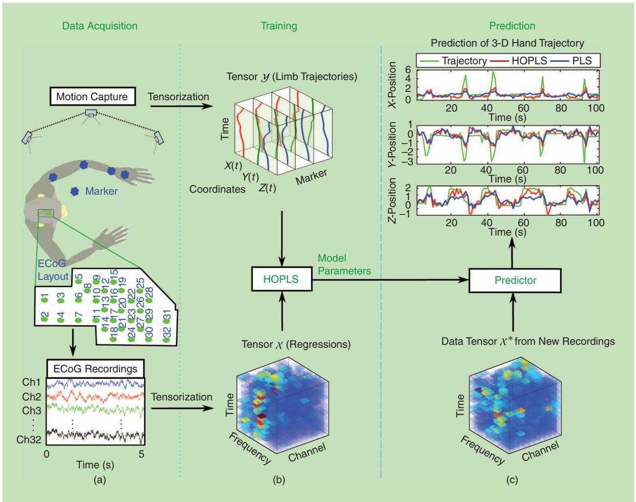
**[FIG14]** The prediction of arm movement from brain electrical responses. (a) The experiment setup. (b) The construction of the data and response tensors and training. (c) The new data tensor (bottom) and the predicted 3-D arm movement trajectories (X, Y, Z coordinates) obtained by tensor-based HOPLS and standard matrix-based PLS (top).
