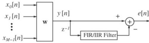
**Fig. 1** BSE architecture based on a linear predictor
