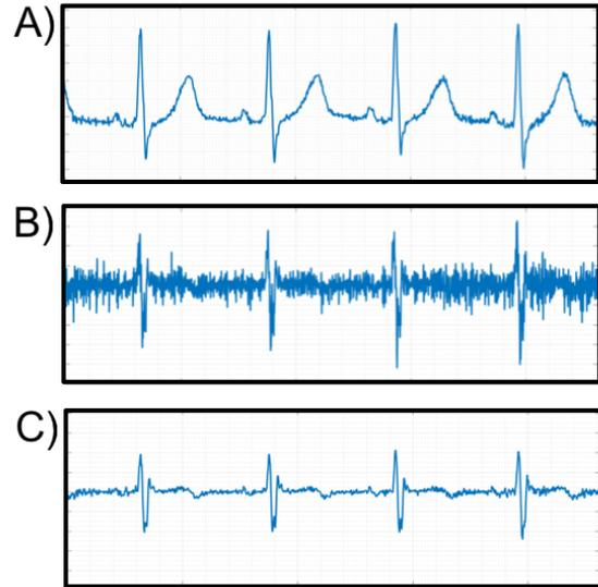
Fig. 5. The effects on ECG of numerical differentiation followed by numerical integration. A) Original ECG signal. B) Numerical derivative of ECG in A) using first order time difference  $x(n) - x(n-1)$ . C) Signal in B after numerical integration using MA filtering.
