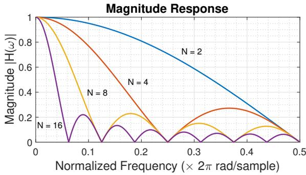
Fig. 3. Frequency response of the MA filter in (1).
