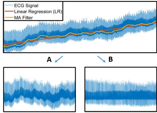
Fig. 4. Baseline drift removal from ECG using linear regression (LR) and a moving average (MA) filter in (1). Observe both the “deterministic” (straight line) and “stochastic” (random local oscillations) component in ECG drift in the top panel. A) Drift removal using LR. B) Drift removal using the MA filter.
