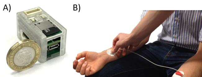
Fig. 1. A) Our iAmp biosignal recording device against one UK pound coin (22.5 mm in diameter). Data can be stored on an SD card or transported in real time to a computer via a mini USB port. B) Placement of electrodes on the forearms for the recording of ECG.
