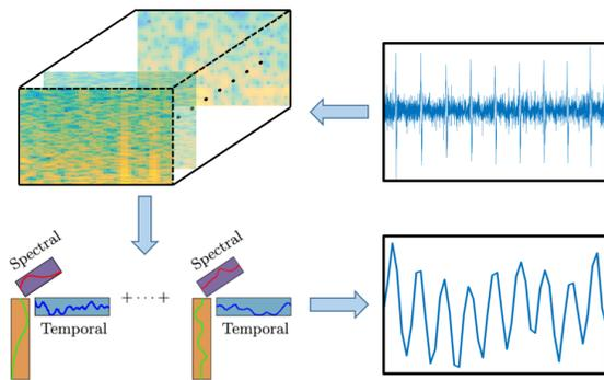
Fig. 6. Using “bio-presence” to teach tensor decompositions for Big Data analytics, an example where Canonical Polyadic Decomposition (CPD) reveals the fundamental periodic pattern in ECG. *Counterclockwise from top right:* First order derivative of the ECG; Data tensor formed by Hankel-folding and STFT; Principle of tensor factorisation using CPD; Fundamental periods in data identified in factor-one CPD (heart rate modulated by respiration).
