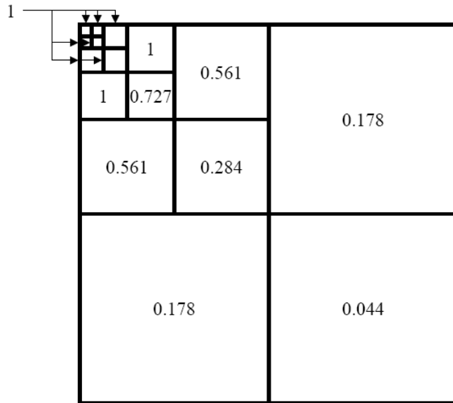
Figure 88 – Possible weighting table for bit allocation
