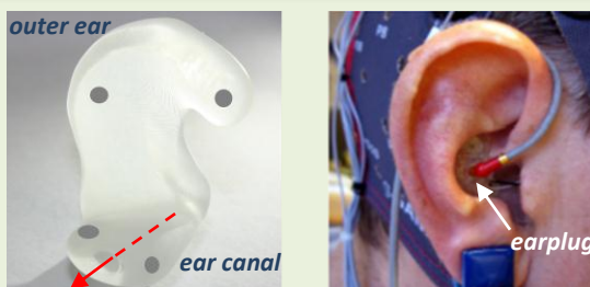
Figure 1: [Left] The left Ear-EEG earplug with electrode positions visible (grey dots) and an arrow indicating the direction in which it enters the ear canal. [Right] Recording setup: joint recording of Ear-EEG and on-scalp EEG for comparative analysis.
