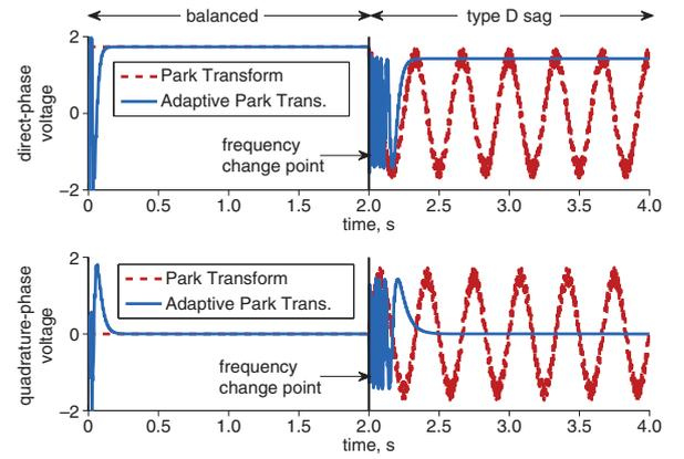
**Fig. 1** Performance of fixed Park transform in (6) and adaptive Park transform in Algorithm 1 under a voltage imbalance and frequency deviation
