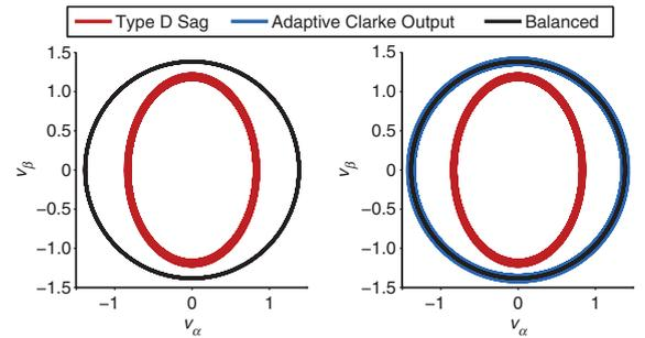
**Fig. 2** Circular profile for  $\alpha\beta$  voltage indicates balanced three-phase system whereas non-circular trajectory indicates a voltage imbalance
