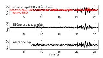
Fig. 4. Motion artefact detection. Top panel: the EEG signal corrupted with motion artefact together with the clean EEG obtained by averaging the signals from four standard electrodes. Middle panel: the difference between the noisy and clean EEG signal. Lower panel: the mechanical output of the multimodal sensor.
