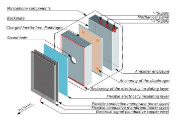
Fig. 1. Detailed construction diagram of the multimodal sensor.
