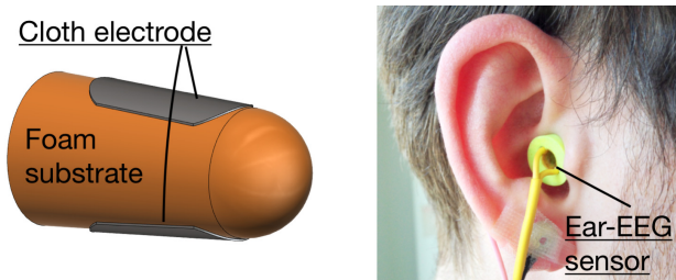
FIGURE 1. The in-ear sensor used in our study. Left: Wearable in-ear sensor with two flexible electrodes. Right: Placement of the generic earpiece.
