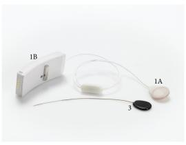
FIGURE 1: Experimental setup. (1A) External disc for power and signal transmission to and from the implanted device. (1B) Logging device to store EEG recorded by implanted device. (2A and 2B) Cup electrodes covered by protecting paper for surface EEG recording. (2C) Ground wire for surface EEG recording. (3) Implantable device with disc for power and signal transmission.
