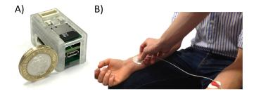
Fig. 1. A) Our iAmp biosignal recording device against one UK pound coin (22.5 mm in diameter). Data can be stored on an SD card or transported in real time to a computer via a mini USB port. B) Placement of electrodes on the forearms for the recording of ECG.
