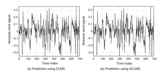
Figure 13.3 The original signal (solid line) and one step ahead prediction (dashed line)
