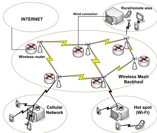
Fig. 1. Typical wireless mesh network scenario.
