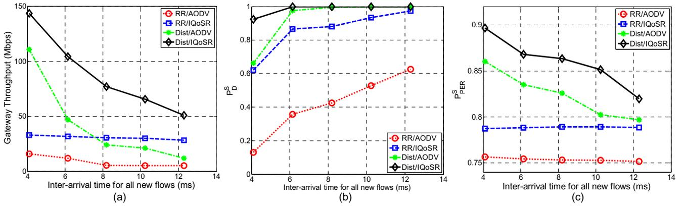
Fig. 2. The effect of network traffic on (a) Network Throughput, probability of successful end-to-end packet reception in terms of (b) Packet Delay and (c) PER.
