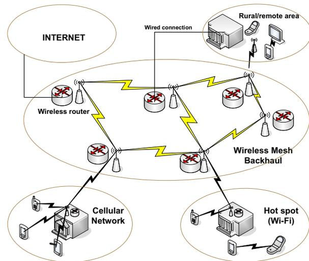
Fig. 1. Typical wireless mesh network scenario.
