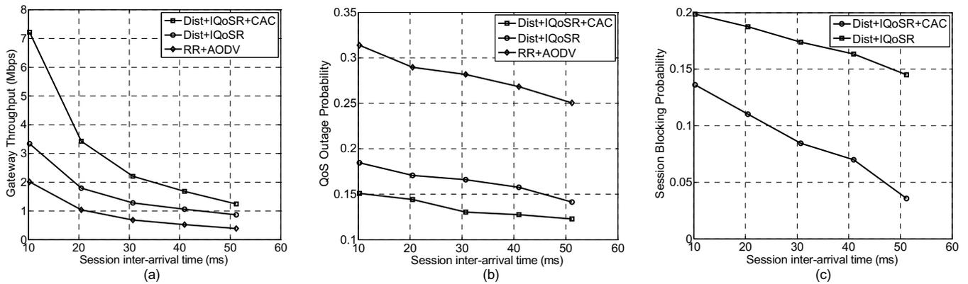
Fig. 2. Simulation results on (a) Network throughput (b) QoS outage probability per session value, and (c) New session blocking probability, all with respect to the new session inter-arrival time.
