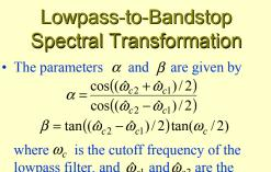
lowpass filter, and  $\hat{\omega}_{c1}$  and  $\hat{\omega}_{c2}$  are the desired upper and lower cutoff frequencies of the bandstop filter
