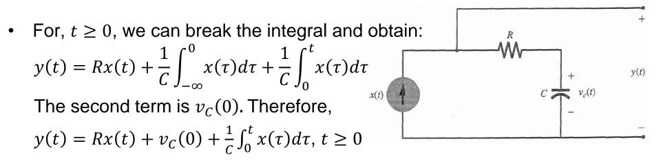
This is a single-input, single-output (SISO) system. In general, a system can be multiple-input, multiple-output (MIMO).
