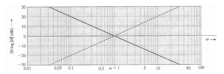
Amplitude responses of a pole (solid line) and a zero (dotted line) at the origin
