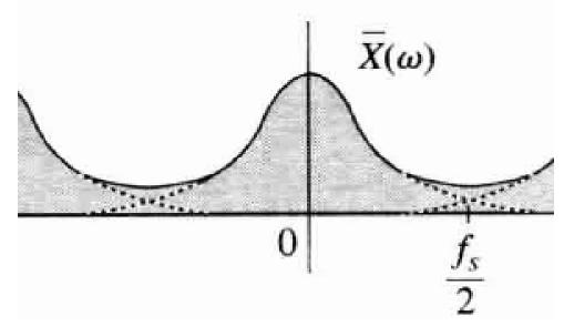
• Furthermore, if x(t) is not time limited, we need to truncate x(t) with a window function. This leads to leakage effect as discussed in previous lecture (sampling).
