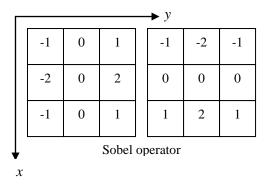
If we consider the left mask of the Sobel operator, this causes differentiation along the y direction. A question that arises is the following: What is the effect caused by the same mask along the x direction? If we isolate the following part of the mask
