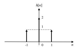
The above response applied to a signal x[n] yields a signal y[n] = x[n-1] + 2x[n] + x[n+1] or in z-transform domain  $Y(z) = (z^{-1} + 2 + z)X(z) \Rightarrow Y(j\omega) = 2(\cos\omega + 1)X(j\omega)$ . Therefore, h[n] is the
